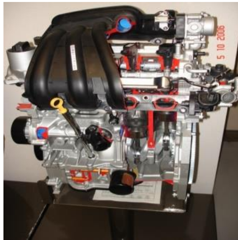
Gambar 1. Mesin DOHC CVTC (Nissan Grand Livina 2007)
